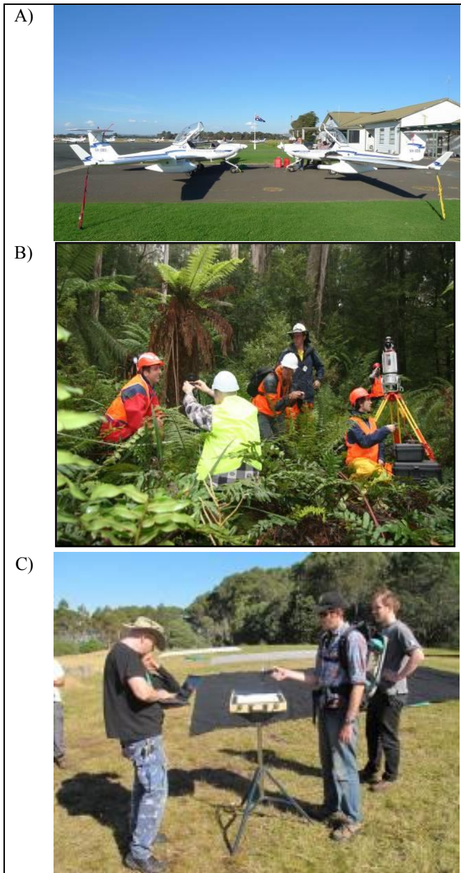
Figure 2. CALVAL associated activities. A) aircraft used to collect high resolution hyperspectral and LIDAR data; B) AusCover CALVAL activities in the Mountain Ash site with participants from RMIT, CSIRO, DSE; C) Ground targets used to calibrate high resolution hyperspectral imagery.
