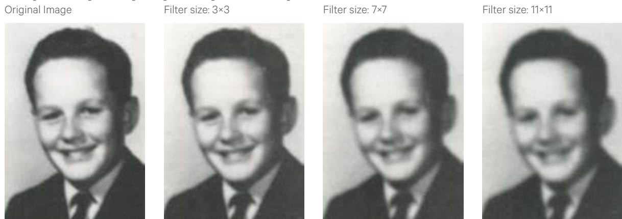
Figure 4.3 Effect of different filter sizes and weights
