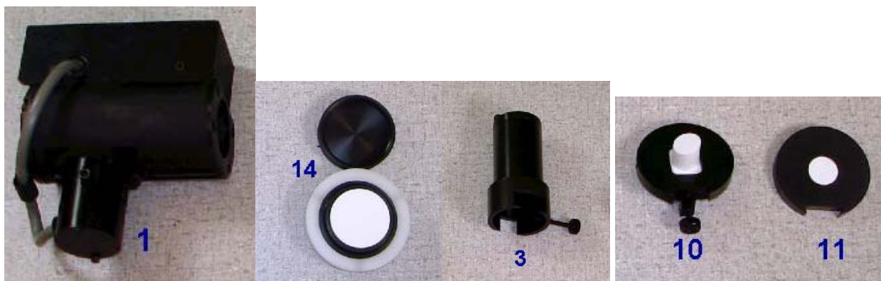
Fig 2. Elements used during reflectance and transmittance measurement procedures. (1) Lamp, (14) White calibrated reference, (3) Light trap, (10) and (11) white reference built-in ports.
