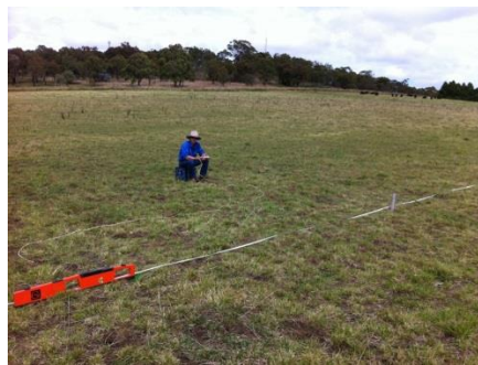
Figure 2. Layout of the measurement transect showing alignment of the EM38 sensor along the 10 m transect and the aluminium (Al) access tube in place.
