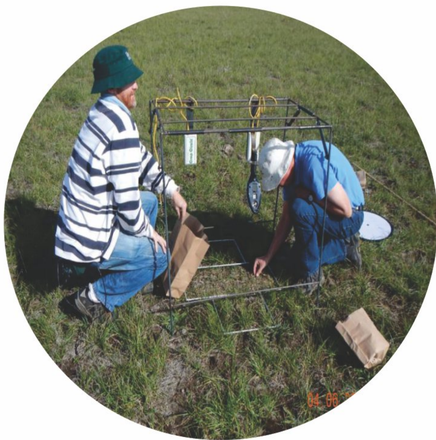
Figure 1. Point source measurement of biomass and corresponding spectral information. All data collection is standardised by using a frame for mounting the Greenseeker hand held and Crop Circle AOS's and a sampling quadrant that encompasses the on ground footprint of both AOS's.
