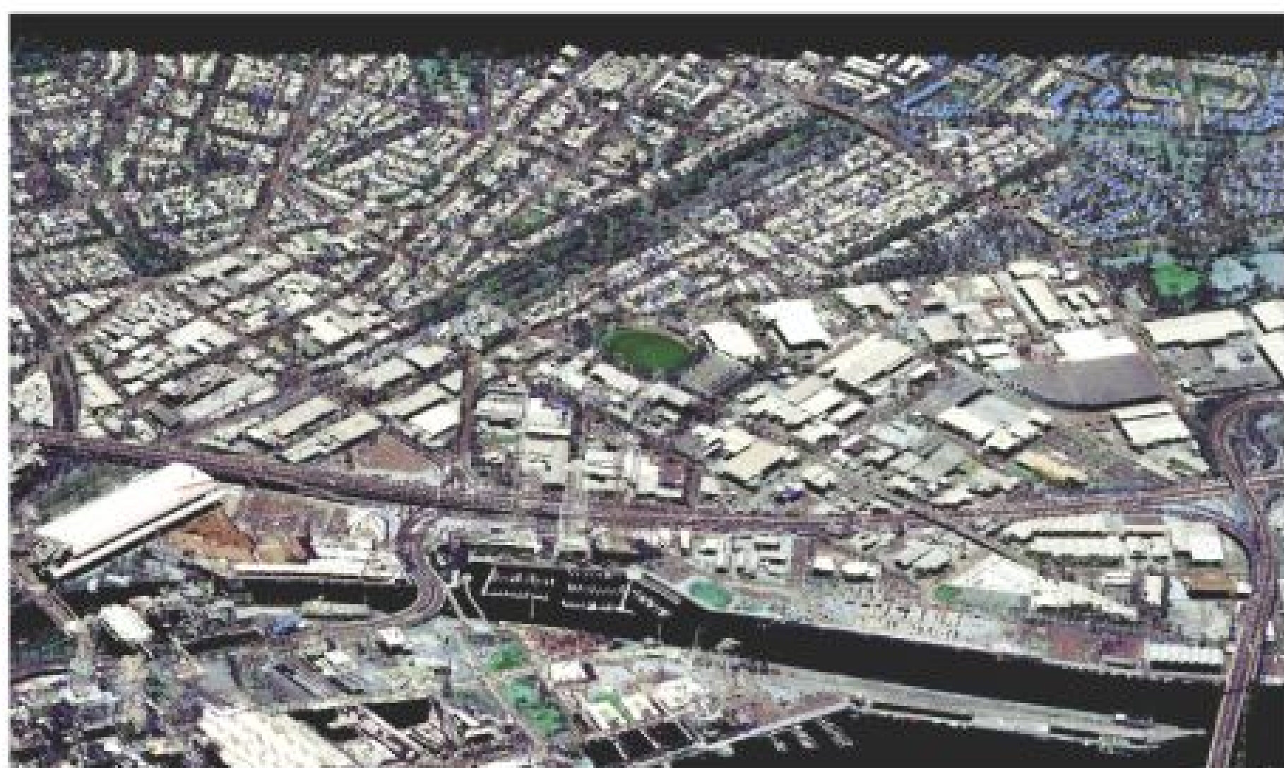
Colourised 3D point cloud
