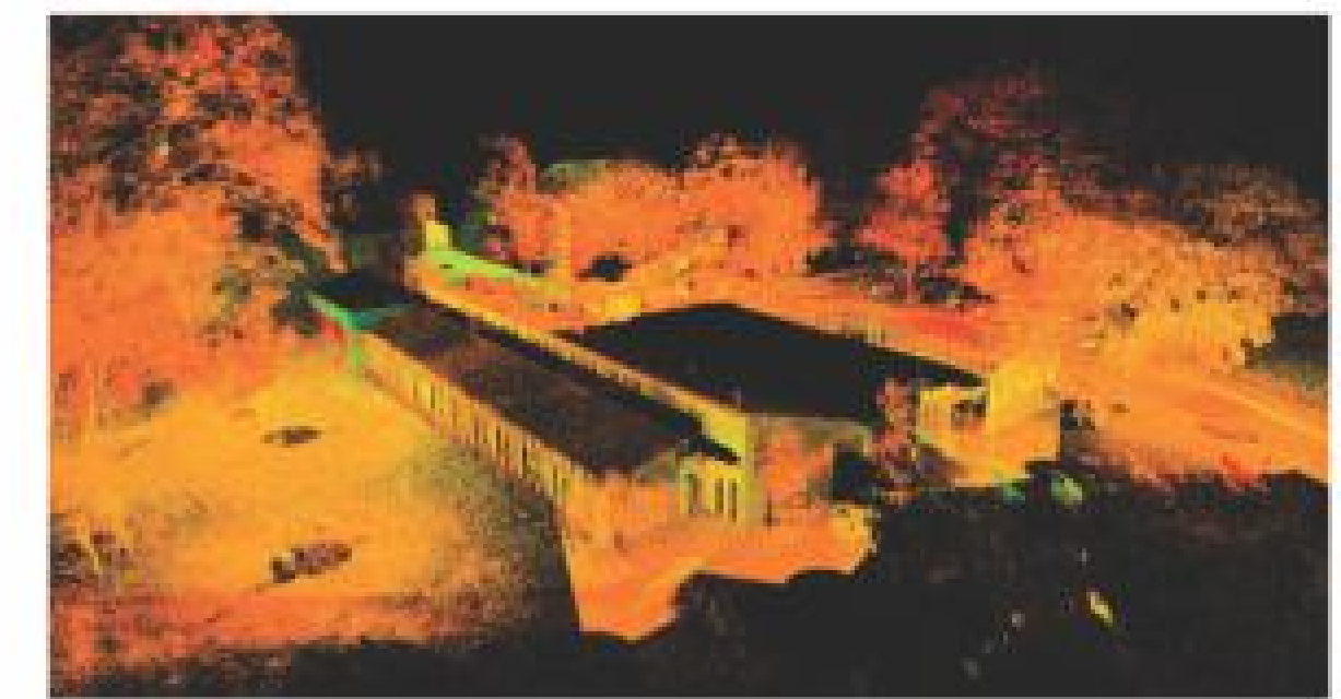
Figure 4: 3D point cloud for the building. Currently the 3D point cloud is used to generate a sketch up description - this generates the DXF file in Figure 5.
