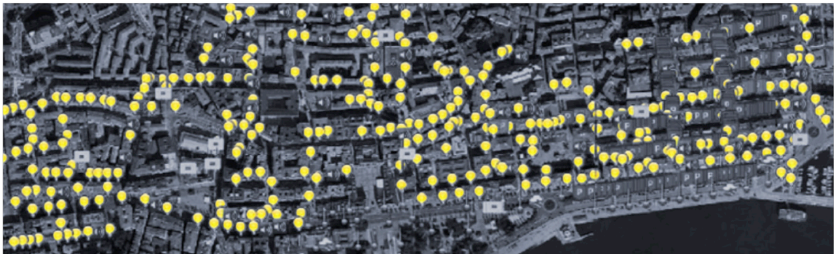
FIGURE 14: THE SPANISH CITY OF SANTANDER, WITH WIRELESS INTELLIGENT MOTES REPRESENTED BY YELLOW PINS
