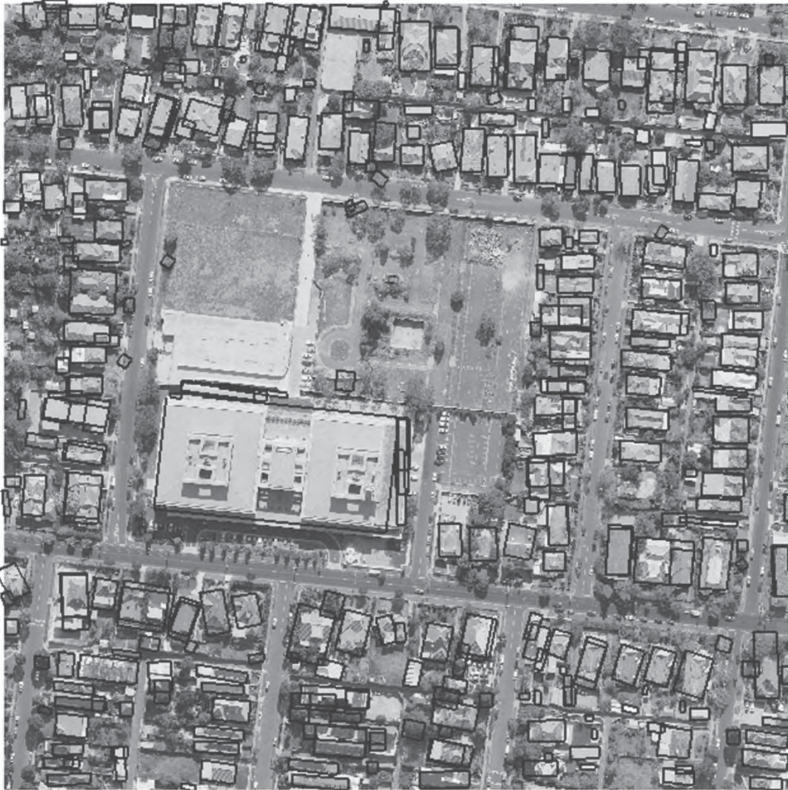
Figure 12. Building detection by the improved algorithm on a scene from Moonee Ponds.
