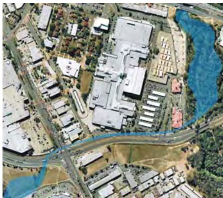
■ Figure B-3. This is a mock up of a possible inundation polygon scenario. The thin part of the polygon is for connection purposes only, no water would be on the surface. Any such thin connecting lines should not be viewed as real surface inundation.
