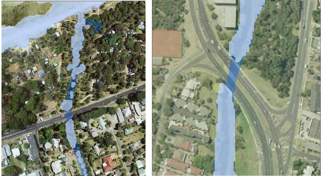
■ Figure 3-2. Left - Remnants of existing vegetation in the ground model cause water blockages in the TINDEM (light blue) but the hydro-enforcement and conditioning process eliminates these anomalies; Right - Bridges not removed from the LiDAR data impede water flow in the TINDEM but after removal in the Hydro-DEM water is allowed to pass through.
