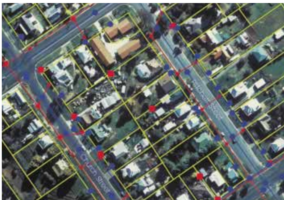
Merged orthophotography, property boundaries (cadaster) and underground services – Sinclair Knight Merz Pty Ltd
