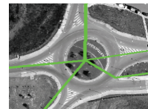
Figure 1. Road vector data overlaid on a high-resolution aerial image.
