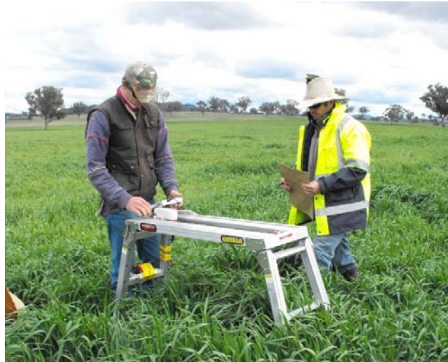
Figure 43 Sliding table fitted with Crop Circle ACS210 in forage oats crop. This is the high biomass site (total > 7,000 kg/ha GDM).
