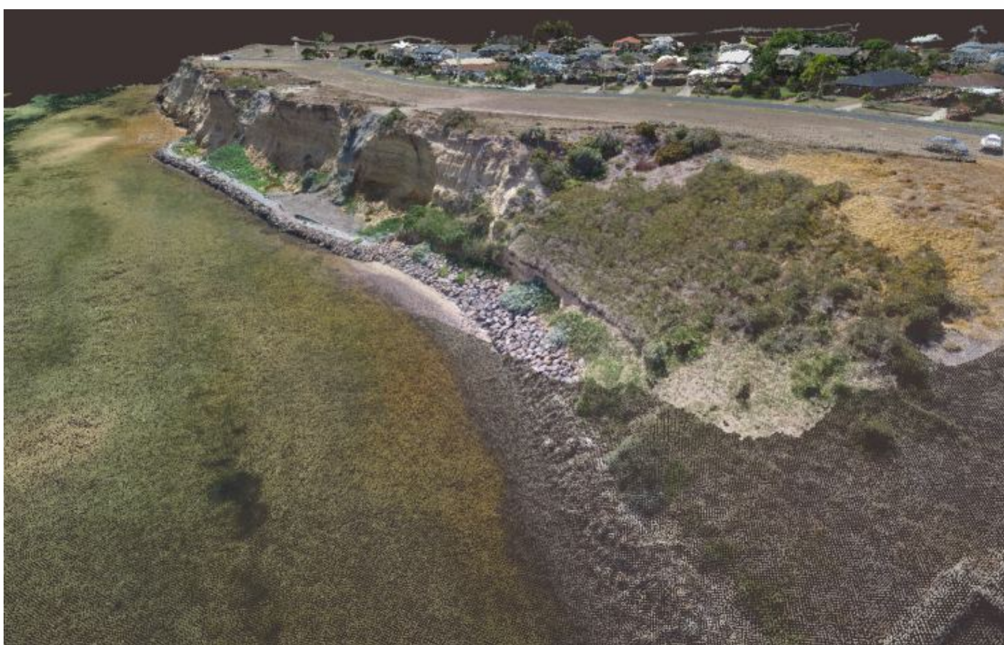
UAV point cloud acquired by Australian UAV using an ebee UAV to capture cliff erosion at Clifton Springs
